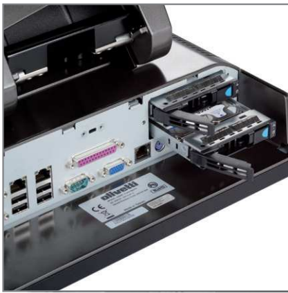
SUPPORT DUAL LAN, TWO REMOVABLE HARD DISK DRIVES AND RAID FUNCTION
